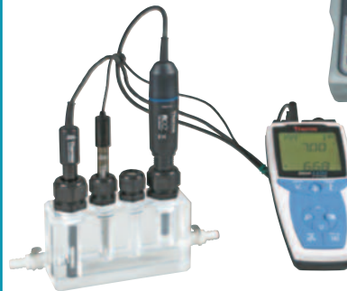
Flowblock A with Thermo Orion Star Series RDO meter and probes installed
