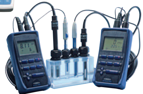
Flowblock A with WTW meters and probes installed
