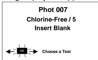
Place a **BLANK TUBE** (sample only) in the test chamber, then press [OK].
