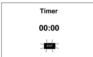
Key in the time required in minutes and seconds, maximum 29 minutes and 59 seconds, using the numerical keys, then press **[OK]** to start the timer. Use the **◀** and **▶** keys to reposition the cursor and re-enter the time if it is keyed in incorrectly.
