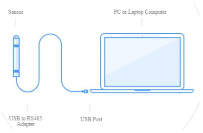
Step 3—Open Aqua4Plus 2.0, software will automatically detect your com port settings and scan for sensors
