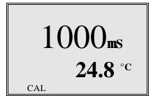
Value of calibration solution at 25°C
