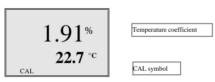
3. Use the **UP ARROW** or **DOWN ARROW** key to change the value to the desired new temperature coefficient.
