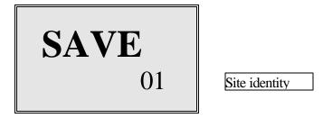
The meter will flash **SAVE** on the display along with the current site identity is being used.
