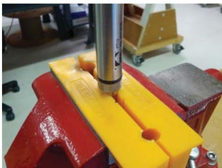
Cabled Sensor - gripping on swage
