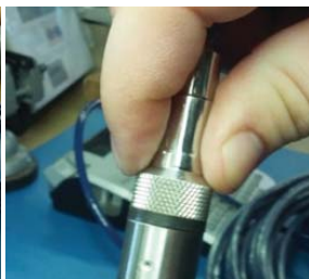
Properly completed — black ring uncompressed
