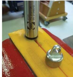
*Cableless Sensor - gripping on knurled area*
