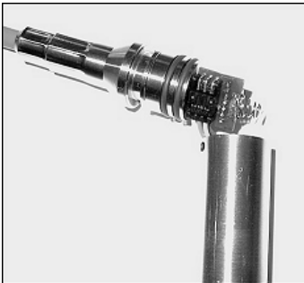
Changing Batteries in Tube Version
