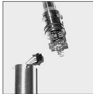
Changing Batteries in Tube Version
