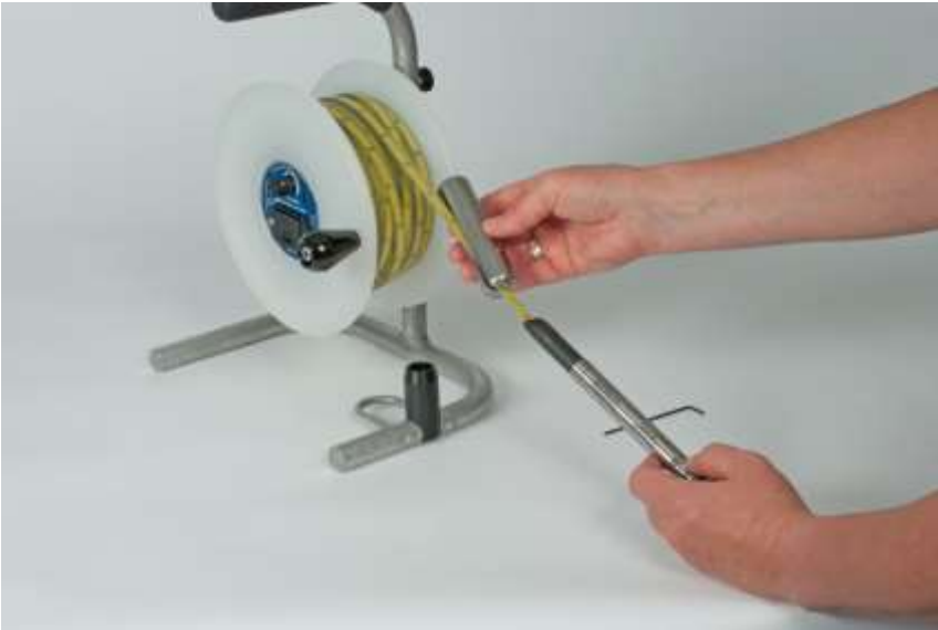
Figure 2-2 Fitting (Optional) Tape Weight
