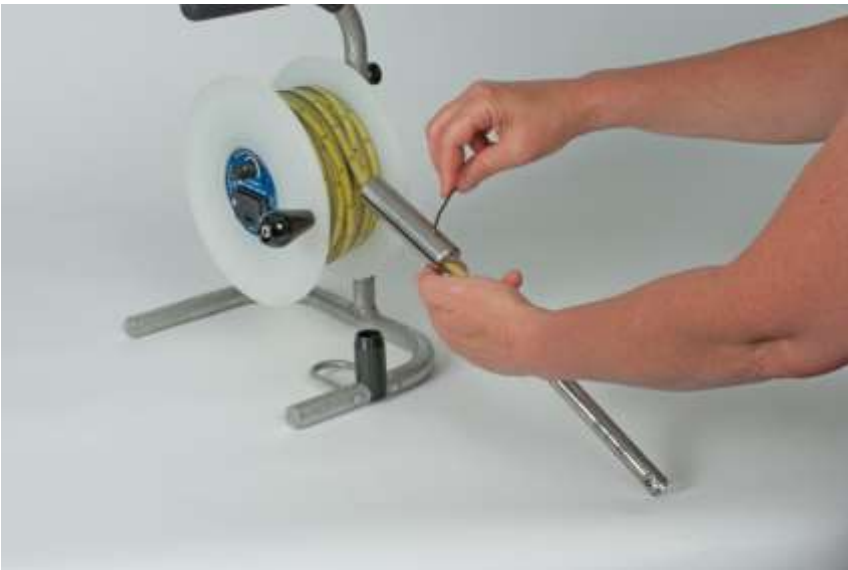
Figure 2-3 Tightening (Optional) Tape Weight
